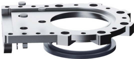
6. The valve body, disc, seals, and packing can be made from corrosion-resistant and wear-resistant materials to address the challenges of abrasive and corrosive slurry. 7. The valve disc has guide sliders on both inlet and outlet, ensuring that the disc remains centered within the valve body during circulation. This guarantees a tight seal and avoids disc scratching by the body.
